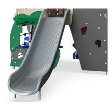
Molded PE slides made with 33% postconsumer materials in different colors in onepiece design with a wall thickness of minimum 5mm. The PE is tested for UV stability and has excellent impact strength and it is usable within a large temperature span.
