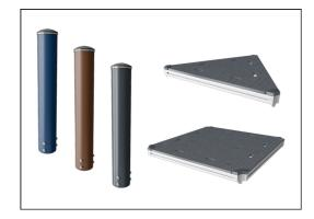
The main posts are made of high quality pregalvanized steel with powder coated top finish. Post tops are closed with caps of UV stabilized nylon (PA6). The grey colored molded decks are made of 75% post-consumer waste PP material with a non-skid pattern and texture surface. All decks are supported by unique designed low-carbon aluminum profiles with multiple attachment options.
