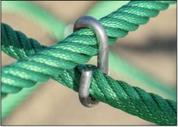
Corocord 'S' clamps are used as universal connections in Corocord products. 8mm stainless steel rods with rounded edges are pressed around the ropes with a special hydraulic press, making them the ideal connector: safe, durable and vandalism-proof, all while allowing the typical movement of rope play structures.
