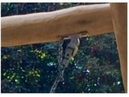
Swing hangers for Robinia wood crossbeams are made of stainless steel brackets and can move over two axis. The flange bearings are silicone enriched to make the suspension maintenance free.
