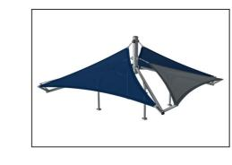
Sails of commercial 95 high density PE knitted specially for sun-shade structures. The sails are treated with UV stabilizers to ensure a long lifetime. The sails are supported by a hot dip galvanized steel frame and tightened by stainless steel devices.
