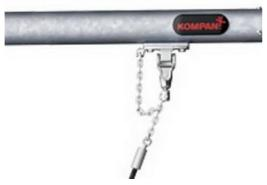
KOMPAN's swing hangers are heavy-duty and designed with stainless steel and anti-twist functions. The hangers attach to the cross beam on a welded bracket with two bolts. The bearings are embedded with silicone lubricant and need no further lubrication; ensuring low maintenance.
