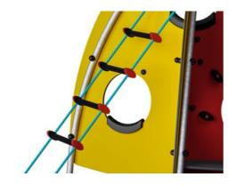
Ropes are made of UV-stabilized PA with inner steel cable reinforcement. The rope is induction treated in order to create a strong connection between steel and rope which leads to good wear resistance.
