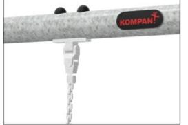
KOMPAN heavy duty designed swing hangers of stainless steel with anti-twist function. The hangers are attached to the cross beam on a welded bracket with two bolts, The bearings are embedded with silicone lubricant and needs no further lubrication.
