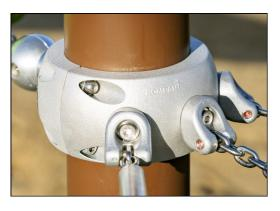
The Corocord Smart Clamps are carefully designed to ensure superior flexibility in high-quality aluminum material. The smart clamps are attached around the post with four steel bolts. Unused attachment points are closed with PA caps.
