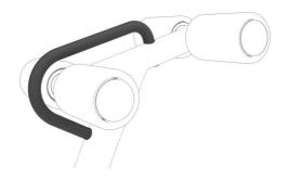
The bench has a support handle with a diameter of ø30mm. The support handle will make it easier to get on and off the bench and it will allow a variation in exercises. The grip powder coating, used on the support handle, is highly durable against wear and tear, offers isolation, and simultaneously gives users an outstanding grip during their workout.
