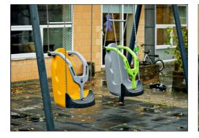
The inclusive swing seat made of recyclable polyethylene (PE) using 33% post-consumer materials. The seat is moulded in one piece and equipped with a drain hole to avoid water accumulation. The ergonomic design enables a safe and comfortable seating position.
