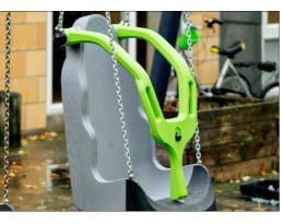
The Harness is made of moulded recyclable polyethylene (PE) made from 33% postconsumer materials. The harness utilises a stainless-steel torsion spring which makes the harness stay in position to secure easier entry and exit of users. The harness lock is designed with a one-handed operation slider made from stainless steel.
