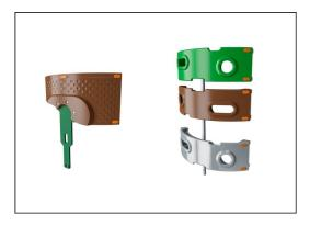
The climbing elements displayed are moulded in one piece with a minimum 5mm wall thickness. The climbing elements are made of recycable PE which has a high impact resistance across a wide temperature span which ensures vandal resistance in all locations.
