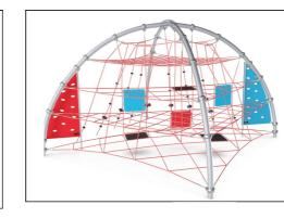
The bended arches are holding the tensioned net structure without additional disturbing fasteners. The arches are produced from high quality stainless steel to allow movement of the net on the surface of the steel arches. The surface is treated to make it shiny.
