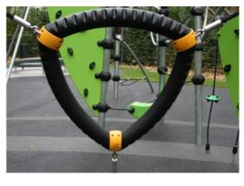
GALAXY climbing triangle with outer soft layer of PUR and corner brackets of moulded nylon (PA6). The core consist of a powder coated welded steel frame with integrated corner suspension points. Larger triangles are closed with an 18mm thick Ekogrip® panel that has a top-layer of rubber with a non-skid effect.
