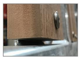
The Wood Plastic Composite panels are made of 100% recycled fibre/wood powder and High-Density Poly Ethylene (HDPE). With the dimensions of 860 x 110 x 30mm the boards are solid.
