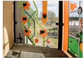
Panels are manufactured from high-quality polycarbonate with a thickness of 15mm. The graphic prints are added by a unique multi-layer print process where the inner layer is the image and outer transparent layer functions as protection. Both PC panel and the water-based lacguer are UV stabilised to prevent fading.
