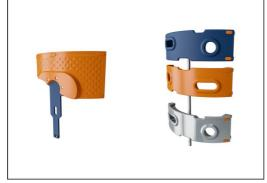
The climbing elements displayed are moulded in one piece with a minimum 5mm wall thickness. The climbing elements are made of recycable PE which has a high impact resistance across a wide temperature span which ensures vandal resistance in all locations.
