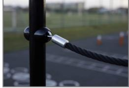
Ropes are made of UV-stabilised PES with inner steel cable reinforcement. The polyester yarn is made from +95% post-consumer materials and is inductively melted onto each strand, leading to good wear resistance.
