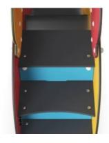
The steps are made of High Pressure Laminate HPL with a thickness 17,8mm and non skid surface texture according to EN 438-6. KOMPAN HPL has high wearing strength to ensure long lifetime in all climates.
