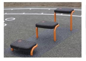
The support frame is ø48.3 x 4mm, carbon steel, with a hot-dip galvanised surface according to ISO1461, and a powder coating corrosion class C3 according to ISO12944-2. Lead content for surfaces are below 90ppm.
