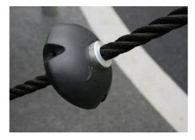
GALAXY Ropes consist of six-stranded steel wires with a steel wire core. Each of the six steel strands is tightly wrapped with PES yarn, which is then melted onto the steel wires. The PES yarn is made of +95% post-consumer materials, allowing it to be highly resistant to wear and tear.
