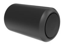
The rotating rollers are Ø 110mm and made from PUR (Polyurethane Rubber, compact foam). The rollers have a steel insert that is electro galvanized. They provide support and ensure a comfortable position. All Steel components are made from carbon steel, with a hot-dip galvanized surface according to ISO1461, and a powder coating corrosion class C3 according to ISO12944-2. Lead content for surfaces is below 90ppm, and below 100ppm for base material. SUD TUC SUD FIL SU
