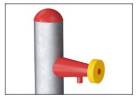
The integrated water tap open for water when pushed and stops when letting go. The water is supplied trough a pipe located inside the post with hose or pipe connection at the bottom of the post. The supply can either be a loose hose or a permanent in-ground pluming.
