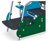
Platform and seats are made of HPL with a thickness of 17,8mm with a very high wearing strength and a unique KOMPAN nonskid surface texture.
