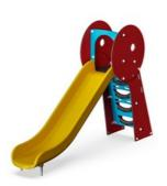
Molded PE slides made with 33% postconsumer materials in different colors in onepiece design with a wall thickness of minimum 5mm. The PE is tested for UV stability and has excellent impact strength and it is usable within a large temperature span.
