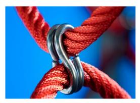
Designed to allow the typical function of rope play structures to move Corocord 'S' clamps are used as universal connections in Corocord products. 8mm stainless steel rods with rounded edges are pressed around the ropes with a special hydraulic press, making them the ideal connector. Our clamps are safe, durable and vandalism-proof.
