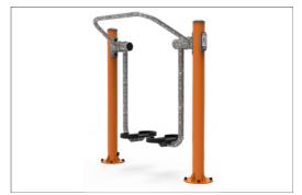
The arms for the foot pedals are 855mm long, and made from ø48,3x4mm S235JR hot dip galvanized steel tube.
