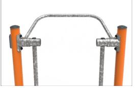
Safety bar is made of tubing with a diameter of 38 mm and wall thickness of 2 mm made of steel S235 with a hot dip galvanized surface treatment according to ISO1461 with a lead content below 90ppm for surfaces and for base material below 100ppm and with powder coated top finish.
