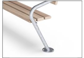
The steel surfaces are hot dip galvanized inside and outside with lead free zinc. The galvanization has excellent corrosion resistance in outdoor environments and require low maintenance. Painted steel parts are hot dip galvanized before powder coating.
