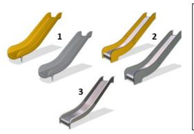
Slides are available in three different materials: moulded on piece PE slides made from 33% post-consumer materials, Combined EcoCore<sup>™</sup> sides and stainless steel slide bed t=2mm. Full stainless steel AISI304 t=2mm. The main posts are equipped with hot dip galvanised steel footings. The steel footings elevates the posts 20mm from ground level to avoid contact with surfacing material.
