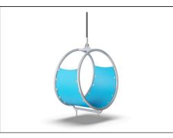
Handout pod designed with a welded frame of two steel rings which are hot dip galvanized and powder coated. The membrane consist of friction-proof rubberized material of conveyor belt quality with excellent UV resistance.
