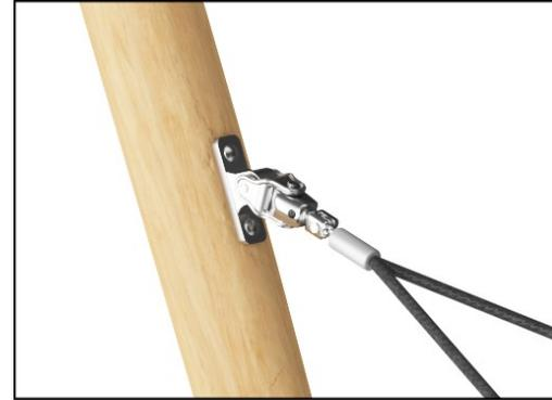
The swing hangers are made of stainless steel brackets and can move over two axis. The flange bearings are silicone enriched to make the suspension maintenance free. At the rope fixation there is a turnable anti twist functions that prevents winding up the ropes.
