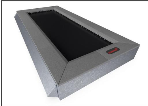
All steel components are manufactured from carbon steel S235 in a thickness of 3 mm. Side panels, support walls for top frame, plates bended with SBR and plates flat for in-situ surfacing are hot dip galvanized. The two long side panels are electro galvanized and powder coated.
