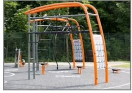
To ensure the integrity of the mainframe is maintained, the orange coloured main posts are made of ø101.6 x 3mm steel posts, which are hot-dip galvanised and powder coated in a variety of colours options. The supportive posts receive the same surface treatment and are made of ø76.1 x 3.6mm steel tubes and finished with coloured powder coating.
