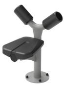
The seat is made of Polyurethane Rubber and has a steel insert plate that is electrogalvanized. The steel plate connects the seat to the frame. This construction makes the seat extremely durable against wear & tear and still very comfortable for a great user experience. The seat is positioned at a height of 46 cm, a comfortable height that makes the transfer from a wheelchair easy.
