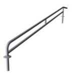
The railing height is 930mm and the distance between the railing is 900mm The material used for the railing is hot-dip galvanized steel ø38 mm, a great diameter for a good grip and wrist support.
