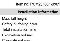
204 cm 46.5 m<sup>2</sup> 23.0 1.16 m<sup>3</sup> Concrete volume  $0.38 \text{ m}^3$ Footing depth (standard) 90 cm Shipment weight 749 kg Anchoring options In-ground
