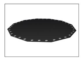
The jumping membranes are made of 6.0mm thick EP Ethylene-Propylene conveyor belt with polyester polyamide fabric carcass. Spring fixations are reinforced with steel bushings and washers on both sides. The membrane is ozone resistant and equipped with 5 center placed water drain holes.
