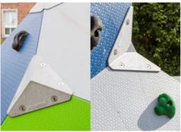
Die-casted corner brackets of high quality lead free aluminium. The corner brackets have nicely rounded edges and countersunk stainless steel screws. For sunny environments the corner brackest can be supplied with optional powder coating which reduced the heat absorption of the brackets.
