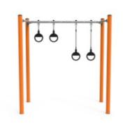
Post are made of Ø101.6 x 2mm, pregalvanized carbon steel and powder coated, a great protection to all conditions. The snake ladder is made of hot-dip galvanized s235 steel with the following dimensions Ø38 x 4mm. The steel surfaces are hot dip galvanised inside and outside with lead free zinc. The galvanisation has excellent corrosion resistance in outside environments and requires low maintenance.
