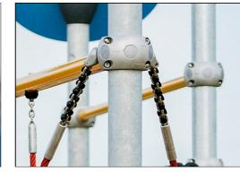
Corocord smart clamps are carefully designed in every detail to ensure superior flexibility in high quality aluminum material. The smart clamps are attached around the posts with four steel bolts. Not used attachment points are closed with PA caps.
