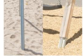
The post of the A-Frame swings is available in two mounting options; surface mounted with anchoring expansion bolts or inground in 60cm or 90cm depth. The hot-dip galvanised steel legs are anchored directly into the ground and Pinewood posts are elevated from the ground by a unique profiled hot-dip galvanised steel footing.
