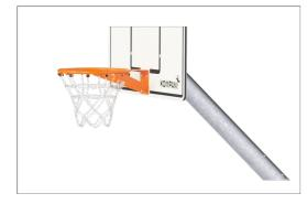
The basketball hoop is made from hot dipped galvanized steel with a powder coated finish. The net is made from Ø4 chain links made from s235 Galvanized steel or stainless-steel chains which meet the requirements in ISO1434-ISO1435 and DIN766. The chains have a circumference of  $\sim$ Ø30cm at the bottom and  $\sim$ Ø50cm at the top.
