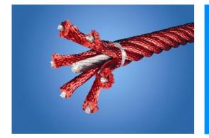
Ropes of UV-stabilized PES rope strands with inner steel cable reinforcement. The polyester yarn is made from +95% post-consumer materials and is inductively melted onto each strand. The ropes are highly wear-and vandalism-resistant and can be replaced at site if needed.
