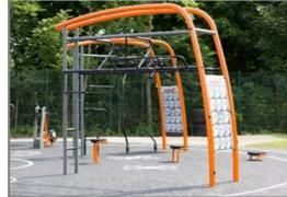
To ensure the integrity of the main frame, the orange coloured main posts are made of ø101.6 x 3mm steel posts, which are hot dip galvanised and powder coated Orange (RAL2010). The supportive posts receive the same surface treatment and are made of ø76.1 x 3.6mm steel tubes, powder coated grey (RAL7012).
