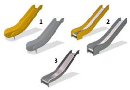
Slides are available in three different materials: moulded on piece PE slides made from 33% post-consumer materials, Combined EcoCore™ sides and stainless steel slide bed t=2mm. Full stainless steel AISI304 t=2mm.
